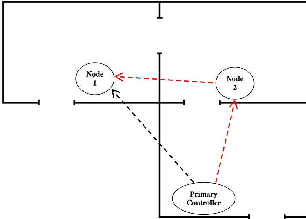
In this example, the message has to pass through two exterior walls in order to reach node 1. There for the calculation will be as follows:
