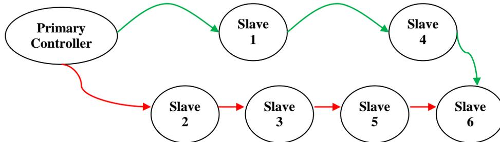
Z-Wave also has an intuitive intelligence where it uses its two-way communication to determine the position of each node, hence may determine the most efficient path is direct communication versus hopping through other nodes.
