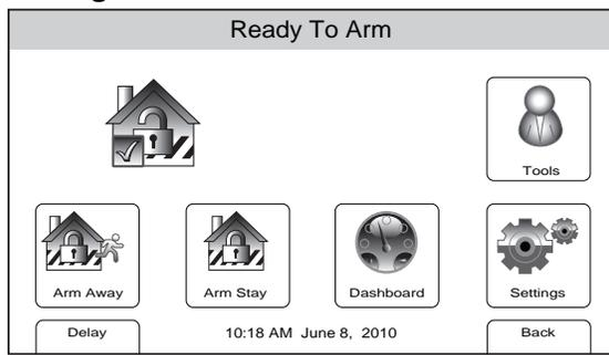
1. With the system in the disarmed state, select the "Tools" icon from the second page of the Home Screen. The system displays the Keypad screen.
