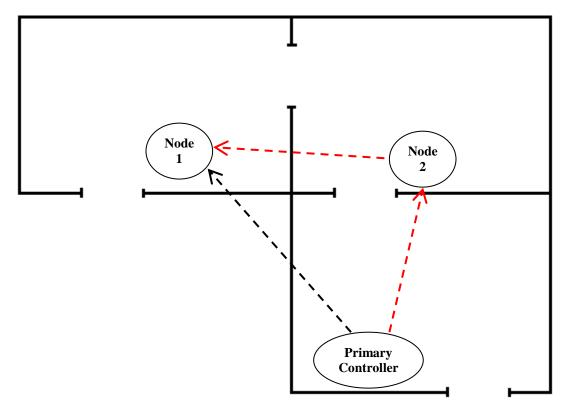
In this example, the message has to pass through two exterior walls in order to reach node 1. There for the calculation will be as follows:
