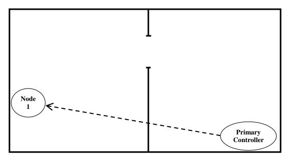
In this example, we have a simple system with one Primary Controller and one Node. For a drywall installation, we calculate the loss as follows:
